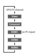
• Pressing [CHANNEL -] reverses the direction of the input modes.
